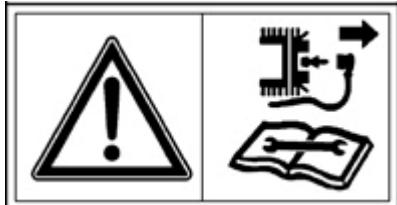
Disconnect the spark plug cap and read the instructions before carrying out any maintenance or repairs!
