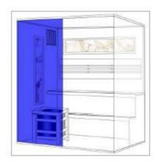
Both solid glass walls (the left part of the FRONT PLATE AND the RIGHT PLATE) must be secured with the included screws with decorative caps to the TOP AND BOTTOM PLATE.
