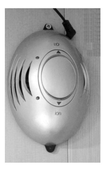
**The ION button** is used to turn on the ionizer. After pressing, the control diode lights up - green.
